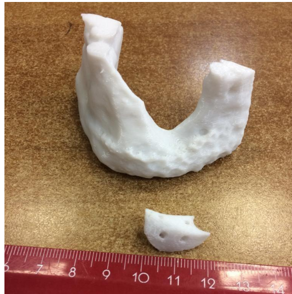
Figure 3. Mock-ups of the jaw and endoprosthesis-expander.
